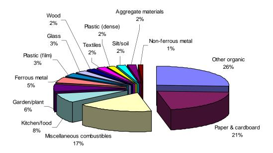
3.4 The above figures shows that, excluding non combustible materials such as metals, inerts and glass, approximately 87% remains potentially suitable for thermal treatment if it is unsuitable for recycling or composting.
