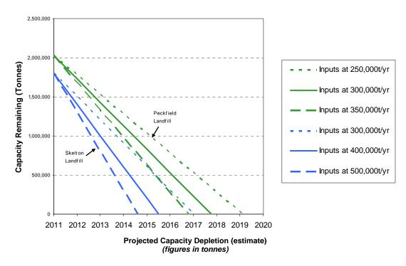
2.13 The diagram above demonstrates the depletion of the remaining void space at both of Leeds' landfills. It can be seen that there will be no remaining permitted landfill capacity for C&I and municipal waste within Leeds after 2019/20.
